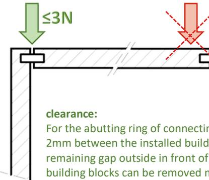
Lasting for weeks uninterrupted too high weight loads can cause flow behavior (deformation) of plastic.
